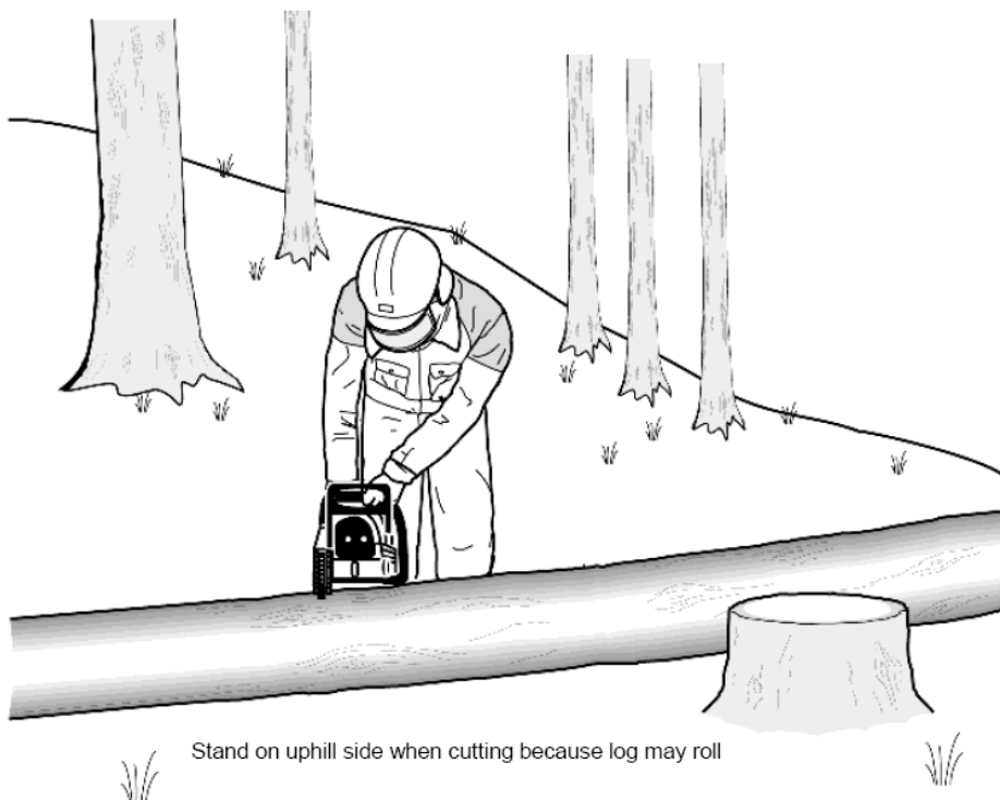
Fig.23 Bucking a log
